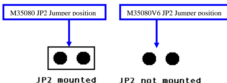
Figure 25. M35080 JP 2 mounted/ M35080 V6 JP2 not mounted
