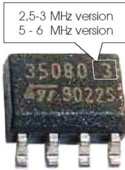
Figure 32. M35080 clock rate index
